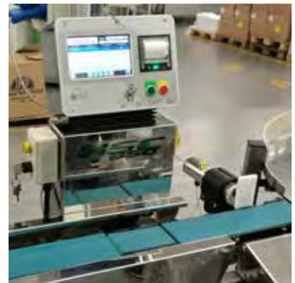
*Double air-blast ejector*
